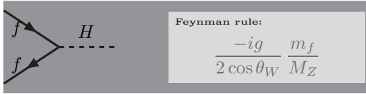
Figure 17.3: Feynman rule for fermion interactions with the physical Higgs boson of the standard model.
