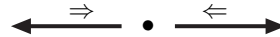
Figure 14.1: Helicity of two fermions produced in the decay of a spinless particle. Each long arrow denotes the direction of momentum of a decay product, and the short one above it denotes the direction of the component of spin along the momentum.
